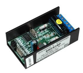
**SMC 81 RP** driver feature small dimensions, step division 1/32, current 1,5A per phase. The driver operation is controlled by small processor RISC. The driver control small and big 2-phase stepper motors with phase current up to 1,5A, providing smooth work of voltage system due step division. SMC81RP driver is installed in U-shaped profile.
